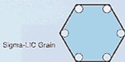
Fujifilm developed Sigma-LIC (Localized Image Centers) Grain technology in order to improve fluorescent light absorption efficiency. It produces silver halide crystals that are flat and hexagonal, with latent image centers concentrated in the corners for increased light absorption. This results in latent images that are more intense and stable than those obtained with conventional silver halide crystals.
