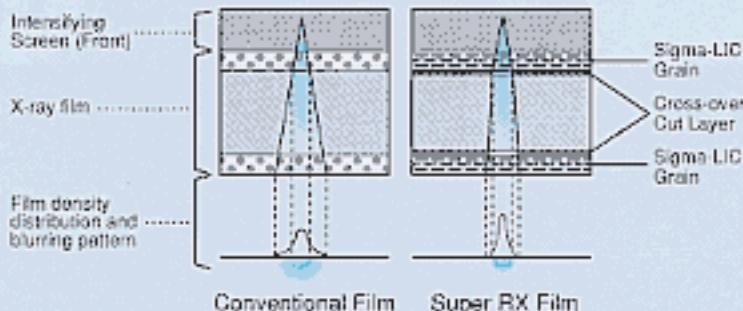
This original Fujifilm technology places ultra-thin layers between the emulsion layer and film base to absorb light. By preventing cross-over light, the extra layers significantly reduce image blurring.
